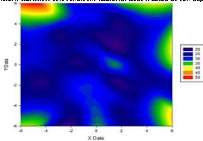
**Fig. 7. Micro-hardness test result for material heat treated at 300 deg for 2 hrs.**
