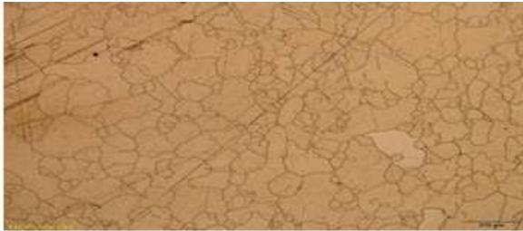
**Fig.1.the microstructure of parent material**
