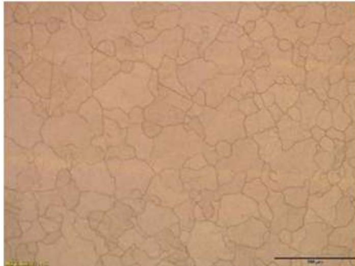
**Fig. 3. The microstructure of material heat treated at 300 deg for 2 hrs**
