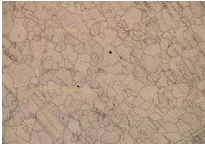
**Fig. 2.The microstructure of material heat treated at 150 deg for 2 hrs**
