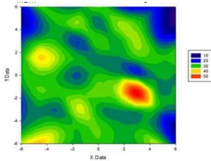
**Fig. 6. Micro-hardness test result for material heat treated at 150 deg for 2 hrs.**
