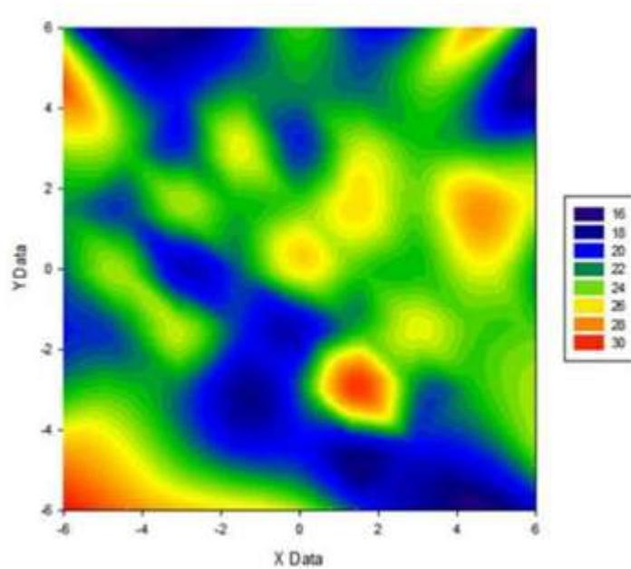
Fig. 8. Micro-hardness test result for material heat treated at 150 deg for 2 hrs.
