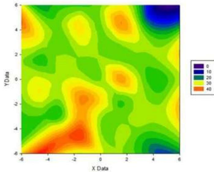
**Fig. 5. Micro-hardness test result for parent material**
